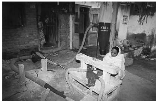
Traditional Grinding Machine with Dust Control System
